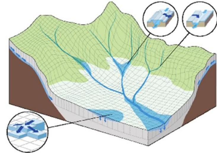
Numerical model for simulation of two-dimensional flood inundation distribution which was developed by ICHARM.
