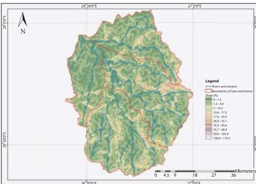
FIGURE 7. Map of the study area showing the average slope (%) of the study site, as computed from the Digital Elevation Model.
