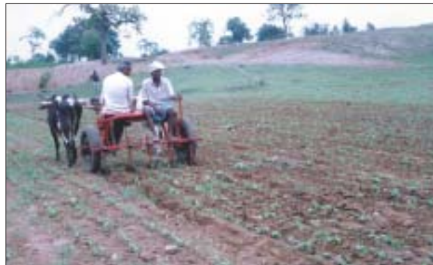
Figure 4. Tropicultor used for planting, fertilizing and covering seeds in a single operation.
